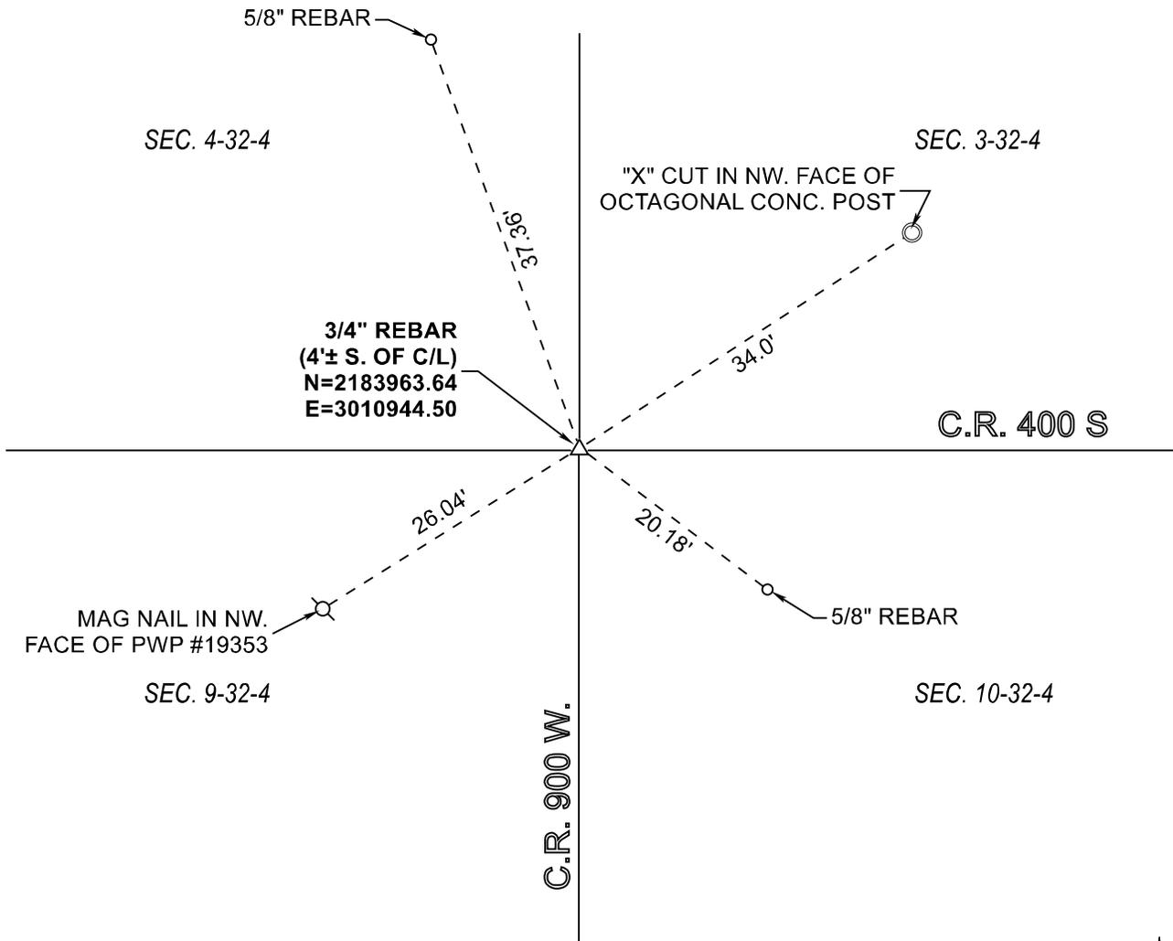
MONUMENT: FOUND 3/4" PIPE IN BAD CONDITION. REPLACED WITH 3/4" REBAR
